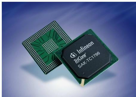
Figure 4 : The 32-bit microcontroller TriCore TC1796 from Infineon [2]
