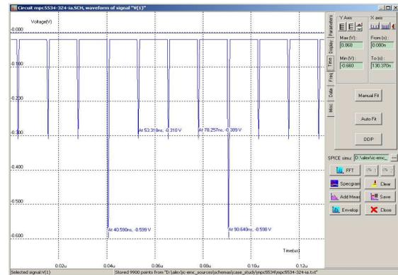
Figure 2: Internal Activity model with a two-phase system, 20 and 80 MHz (mpc5534-324-ia.sch)
