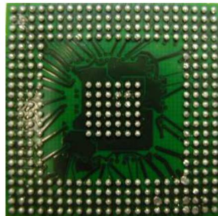
Figure 1 : Bottom side of the 324-pin BGA package of MPC5534
