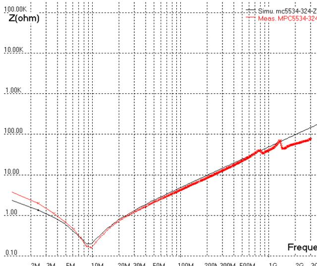
Figure 1:  $Z(f)$  between VDD and VSS of the MPC 5534 BGA (mpc5534-324-ZofF.sch, mpc5534-324-ZofF-Vdd-Vss.z)
