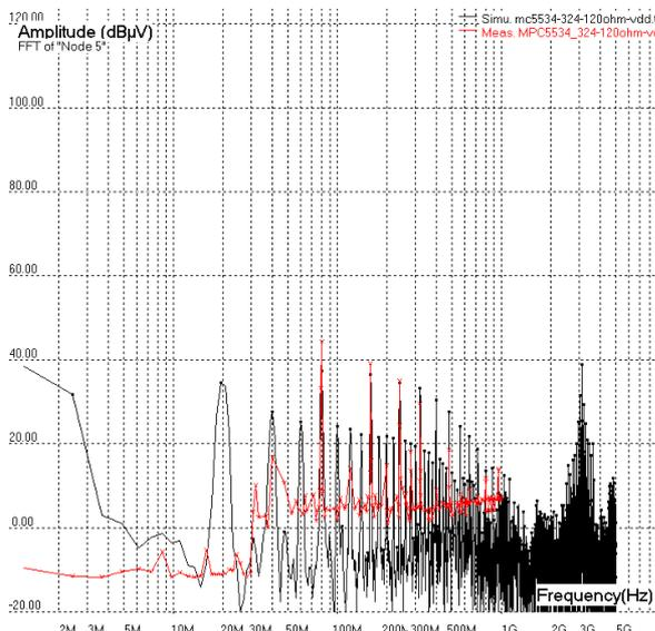
Figure 2: Conducted noise simulation and measurements on the VDD supply rail (mpc5534-324-120ohm-vdd.sch)
