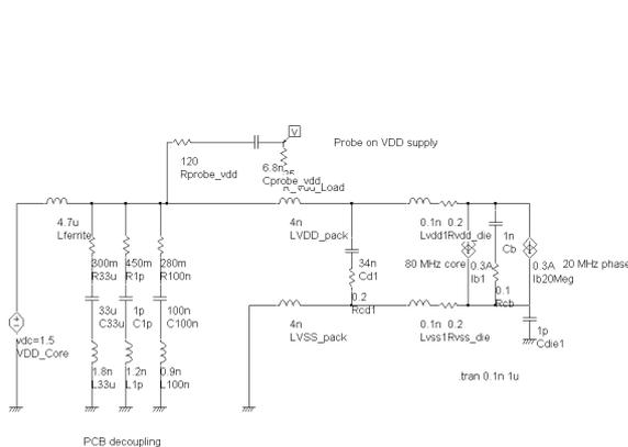
Figure 1: The 120-Ω and 6.8nF probe on VDD supply for monitoring the conducted noise on the VDD supply rail (mpc5534-324-120ohm-vdd.sch)
