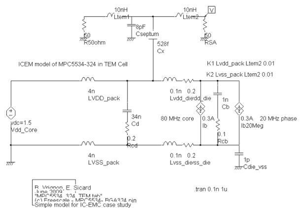
Figure 3: Adding the TEM cell model to the MPC5534 ICEM model (mpc5534-324-tem.sch)
