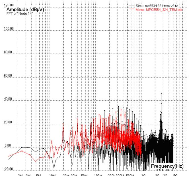
Figure 4: Comparing measured and simulated MPC5534 performances in TEM cell (mpc5534-324-tem.sch, mpc5534-324-tem.tab)
