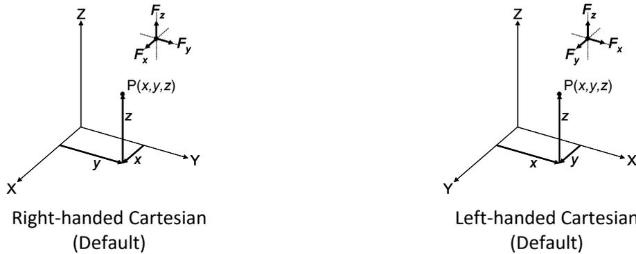
Figure 12 : Cartesian coordinate system definition
