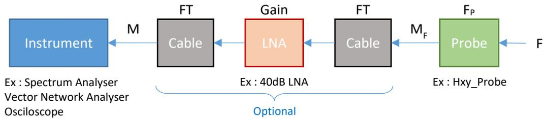
Figure 6 : diagram of setup
